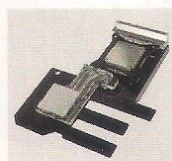
Above: Bitspower's new full-cover motherboard blocks (photo and concept) Below: A full-sized waterblock sits underneath the board for cooling the CPU
